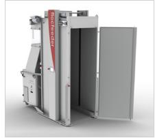
Increase the efficiency and costeffectiveness of the industrial insulation of timber construction elements with the flocfeeder big bale shredder and isofloc cellulose big bales. With flocfeeder, big bales are processed automatically with minimum dead times.
